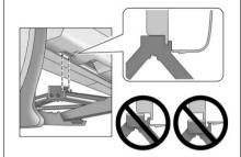
Raise the jack by turning the wheel wrench clockwise until the slots in the jack head fit into the metal flange located behind the V-shaped locating notches on the plastic molding as shown.
